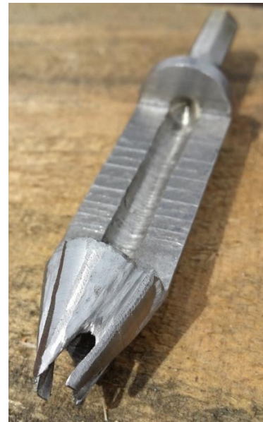
Figure 8. Final prototype made of mild steel.
