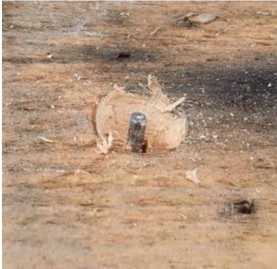
Figure 9. The hole and nail left in the wood from testing with the drill bit.
