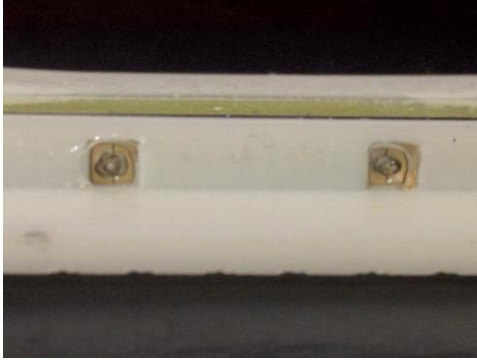
Figure 6. Small slots shown where soldered connections could be placed.
