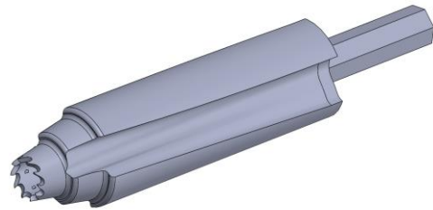
Figure 3. The initial design of the drill bit. The drill bit body was 2.5" long with a maximum diameter of \frac{3}{4} ".
